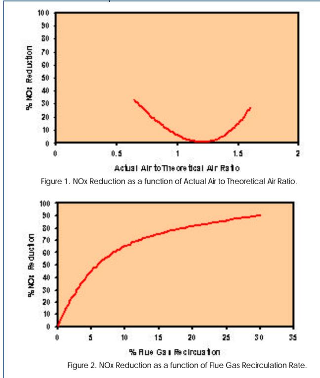
that of SCR! Since the total installed cost of burner systems is an order of magnitude higher than FGR; and, since most of the NOx reduction in the newer burners is due to FGR, the most cost-effective alternative is the proven standalone FGR technology. In a typical FGR application, about 5 to 25 % of the flue gases is recycled back to the combustion zone resulting in NOx reduction as high as 80%.
